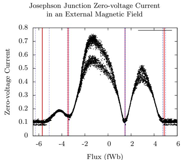
FIG. 7. The flux quantum is measured to be  $3.4 \pm 0.2$  fWb by varying an external magnetic field and measuring the zero-voltage current through a Josephson junction. The flux quantum is the distance between zeros of the smaller peaks.
