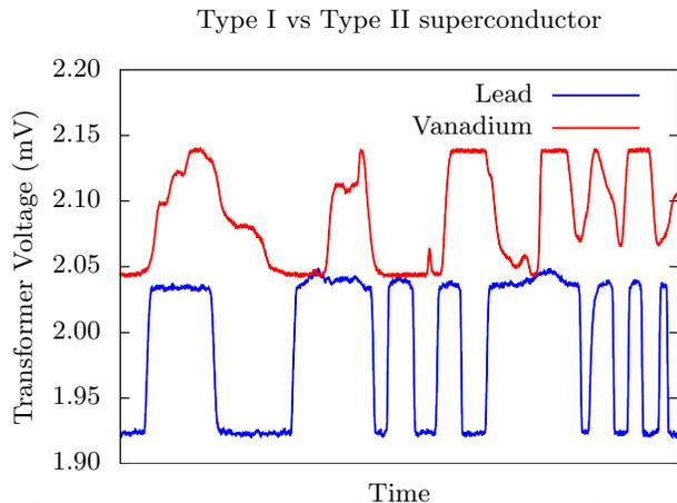
FIG. 2. The transitions in lead, a Type I superconductor, are much sharper than those in vanadium, a Type II superconductor (the temperature modulation was different for the two samples, so the transitions do not line up)
