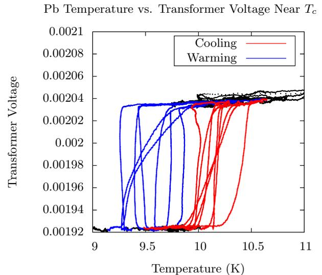
FIG. 3. Examining transitions between the normal and superconducting states of lead reveals hysteresis in the thermocouple-superconductor system
