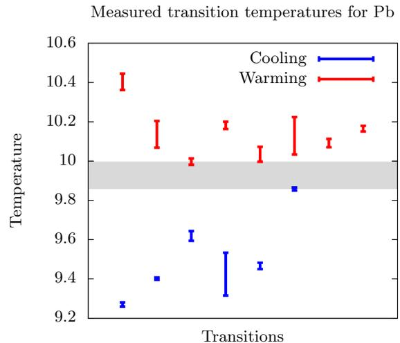
FIG. 4. The real transition temperature can be constrained to be in the gray box, between the coolest warming transition and the warmest cooling transition. The error bars represent the slope of the transition.
