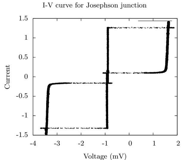
FIG. 6. The I-V curve for a niobium Josephson junction has two interesting features. First, a very high frequency AC current appears when zero voltage is applied. Secondly, no DC current flows until the applied voltage is  $2\Delta/e$ , where  $\Delta$  is the superconducting energy gap.
